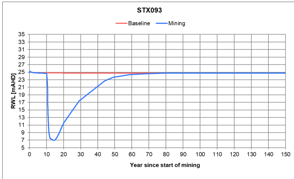
Figure 3-42 Hydrograph showing predicted transient water table response to mine water affecting activities at STX 093 (stygo fauna bore, Type 1 GDE)
